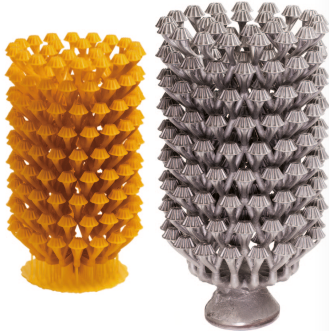
Castable models for industrial use made with DWS 3D printers and materials can be of refined and complex design.
